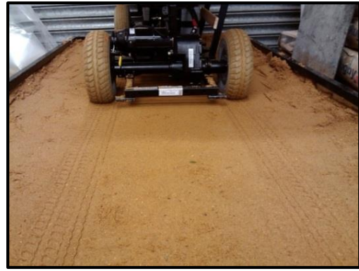
Figure 6: 800N/3PSI combination with minimum rutting and highest traction in the sand bed
