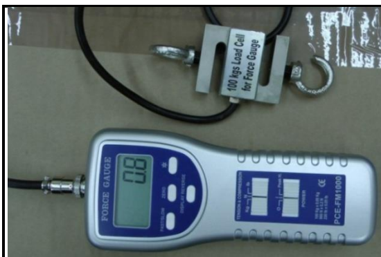
Figure 3: Dynamometer load cell and PCE-1000 force gauge
