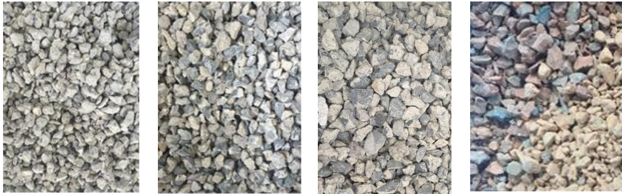
a) RA from laboratory waste b) RA from pavement c) RA from demolished urban buildings d) RA from demolished bricks
