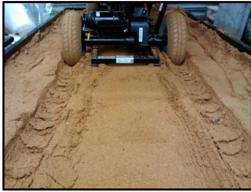
Figure 5: 800N/45PSI combination with maximum rutting and lowest traction in the sand bed
