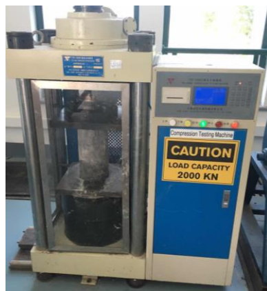
Figure 6: Compressive strength test of concrete cylinders
