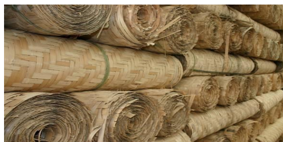
Figure 4: Coarse woven mats form the building stones for BMB (Source: Van der Lugt et al. 2009)
