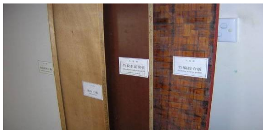
Figure 7: Various kinds of bamboo board material including BMB (Source: Van der Lugt et al. 2009)
