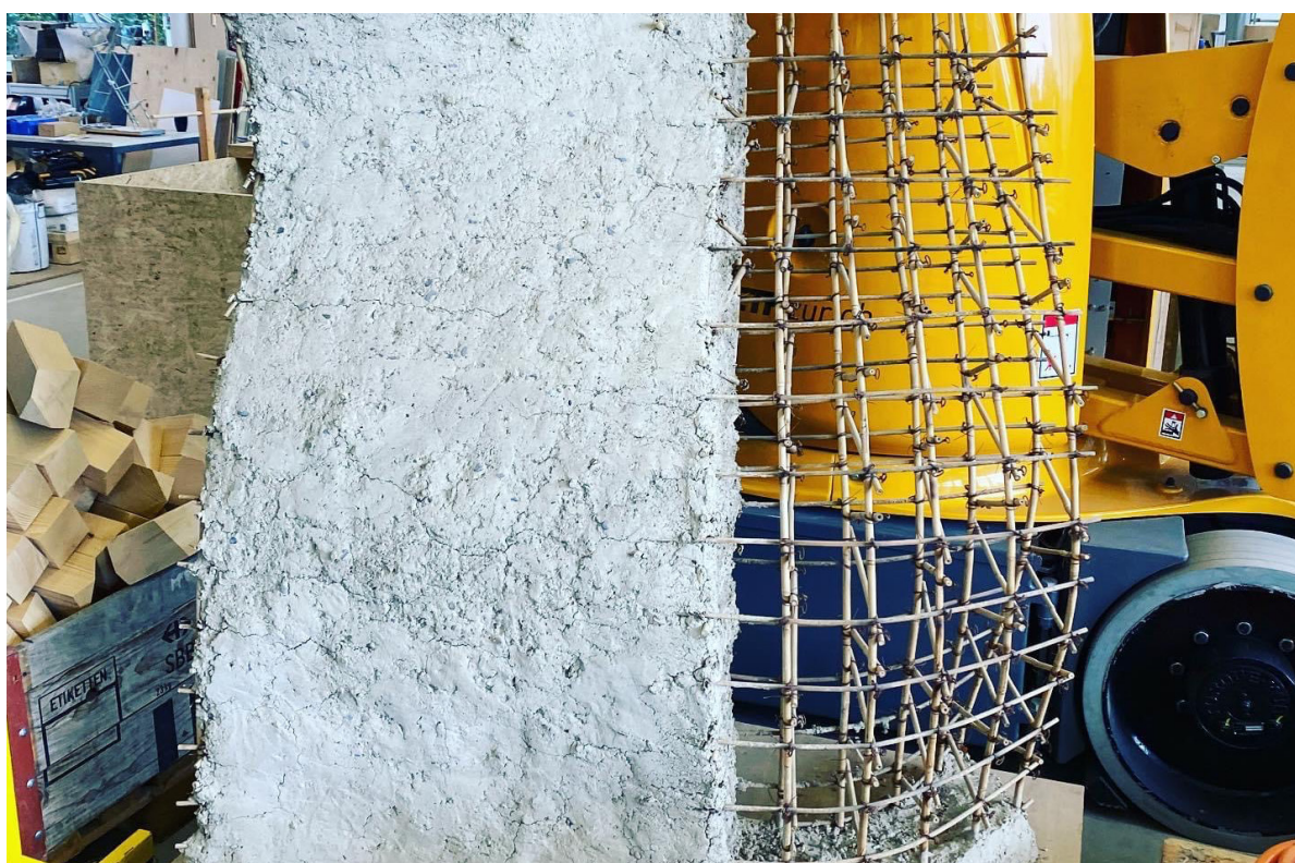
Figure 53: FADA Fablab Anti-shuttering concrete with bamboo rebar.
