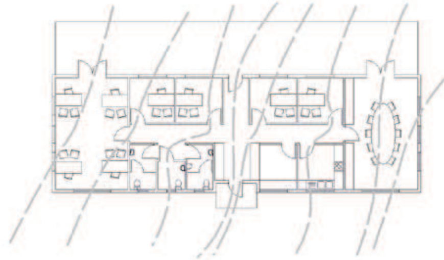
Figure 7. Diagram showing cross ventilation in a building
