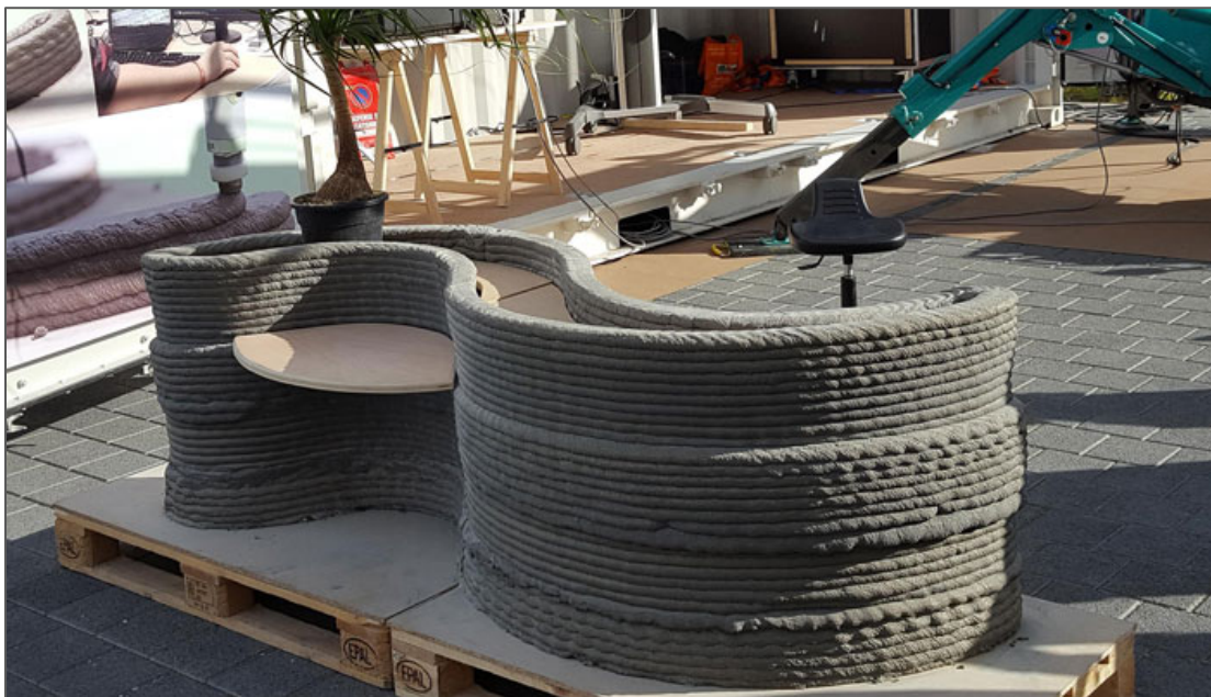
Figure 1.4: Individual layers of cement on a structure created by Constructions-3D
