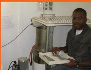
SQUID magnetometer with sample magazine
