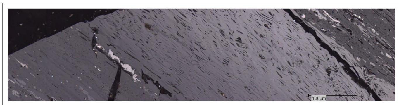
Figure 1: Mosaic photomicrograph showing fusinite (right; well-preserved structure, high reflectance) grading into semifusinite (structured still, lower reflectance), and finally into vitrinite (bottom left; unstructured, lowest reflectance) observed in the inertinite-rich sample. 500x magnification, reflected light under oil immersion. Scale is indicated.
