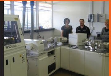
Laser ablation multicollector ICP-MS
