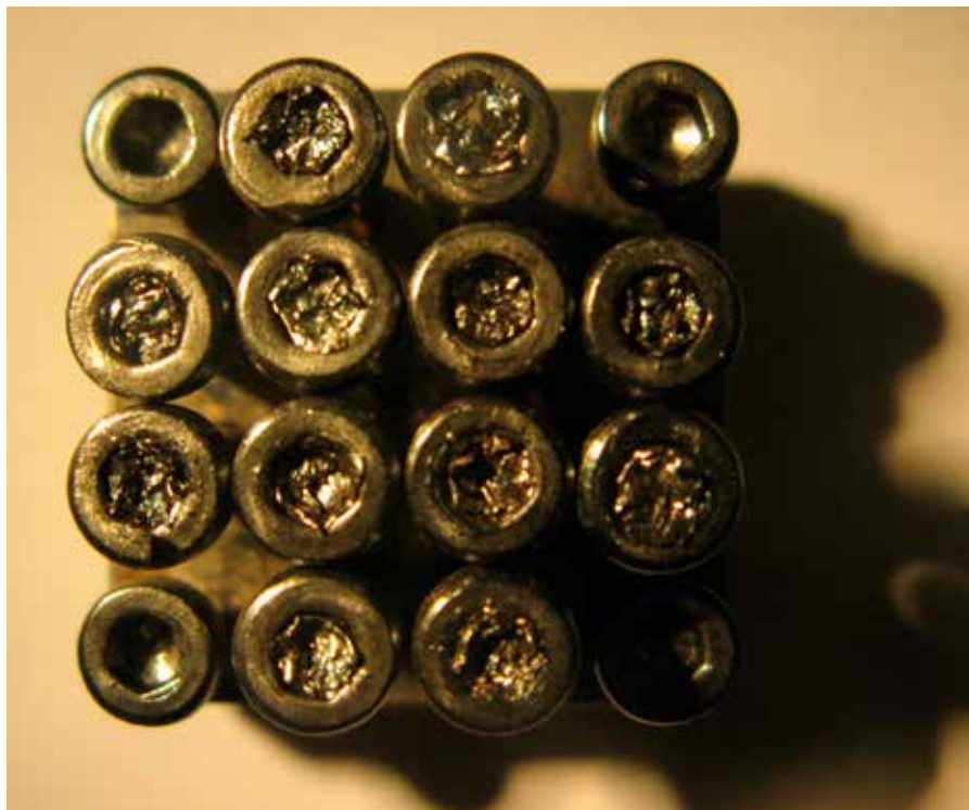
Figure 1. samples encapsulated in copper foil and carbon coated. Internal sample holder diameter is 3 mm.
