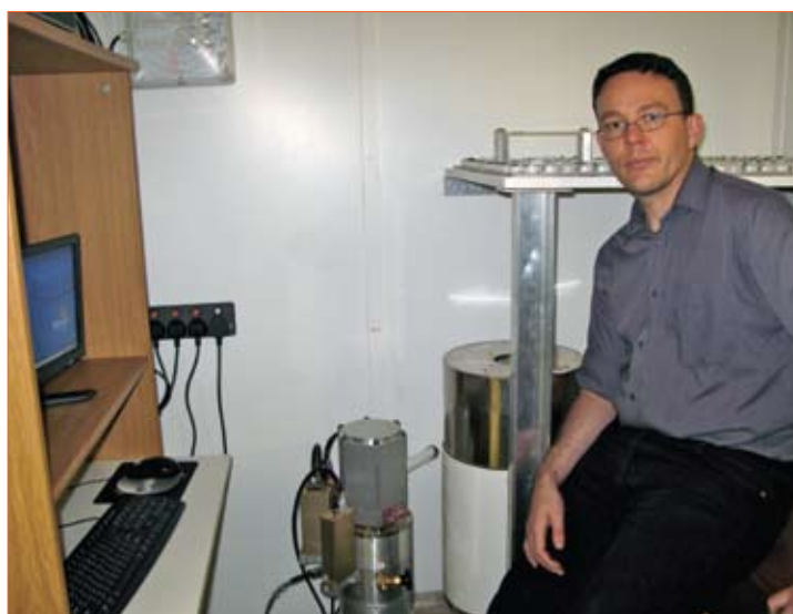
Dr. de Kock in front of “Du Toit”, a vertical 2G Enterprises DC-4K (liquid helium free) superconducting rock magnetometer, and automatic sample changer (designed by Prof Joe Kirschvink of Caltech, USA)
