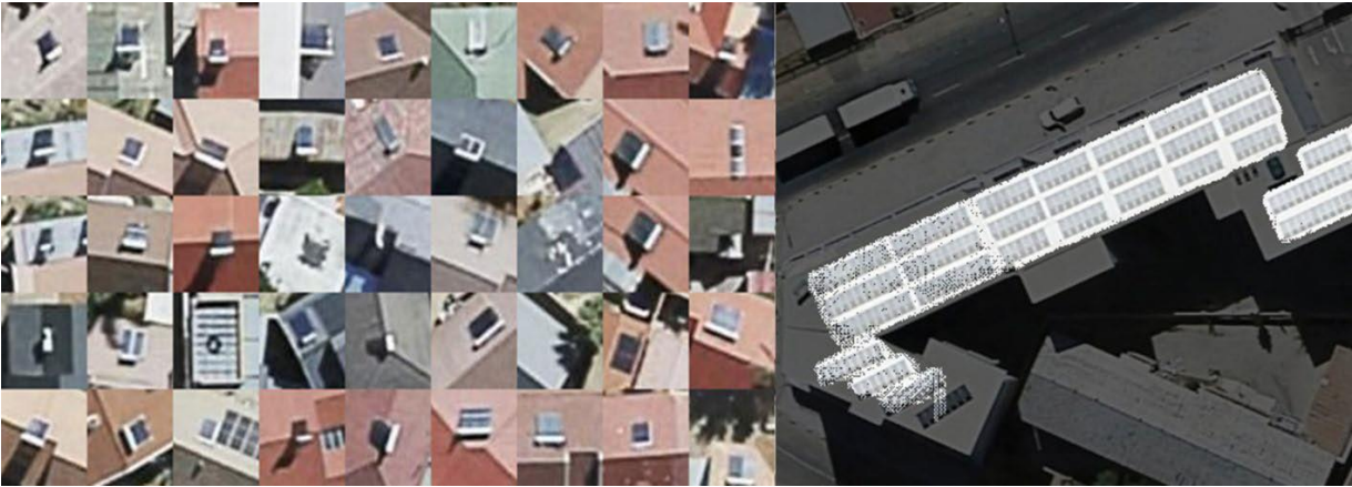
Figure 2 Identified SPV and SWH from aerial imagery.
