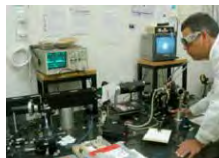
Prof Hearne operating the laser heating facility. Laser hot-spot in the DAC cavity is seen in the background
