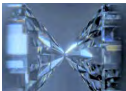
View of a pair of diamond anvils being aligned for experiments.
