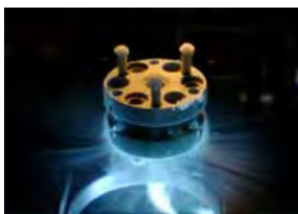
Spectacular picture of one of our miniature DACs warming up, after having loaded a cryogenic pressure transmitting medium into the sample cavity.
