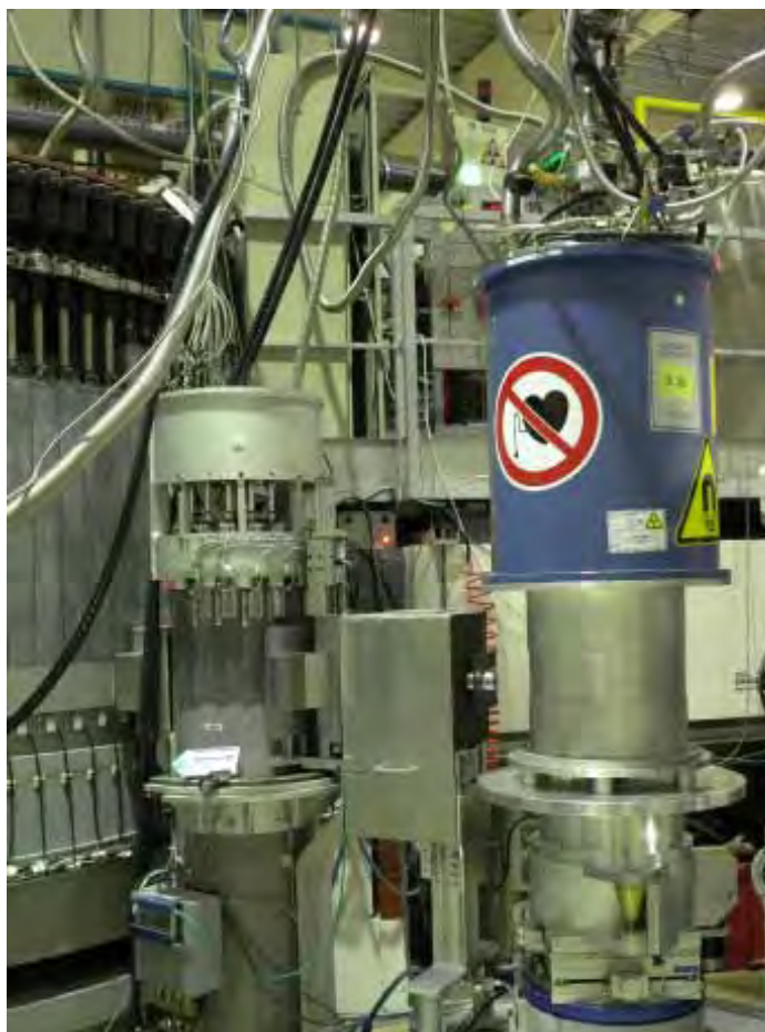
Neutron detectors and cryogenic arrangement on the D23 beamline on the research reactor of the Laue-Langevin Institute, situated on the Isère island on the outskirts of Grenoble (France), where Prof André Strydom recently participated in a Austria-France-South Africa jointly proposed experiment to search for coherent signatures of magnetic ordering in the intermetallic compound \text{Ce}_3\text{Pd}_{20}\text{Si}_6 . This material has the unique feature of quantum criticality in a 3-dimensional crystal structure deep within a quadrupolar electric ordered phase. This is a work in progress and findings are expected to be published soon.
