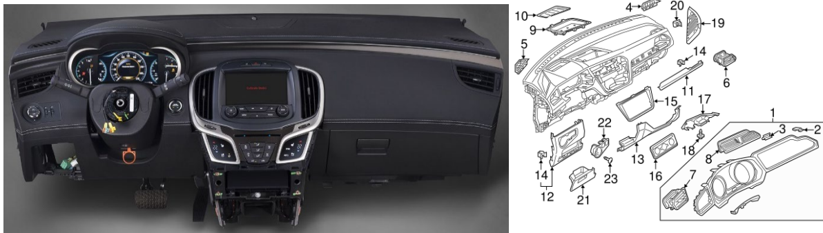
Figure 2: Exemplary instrument panel and its individual components
