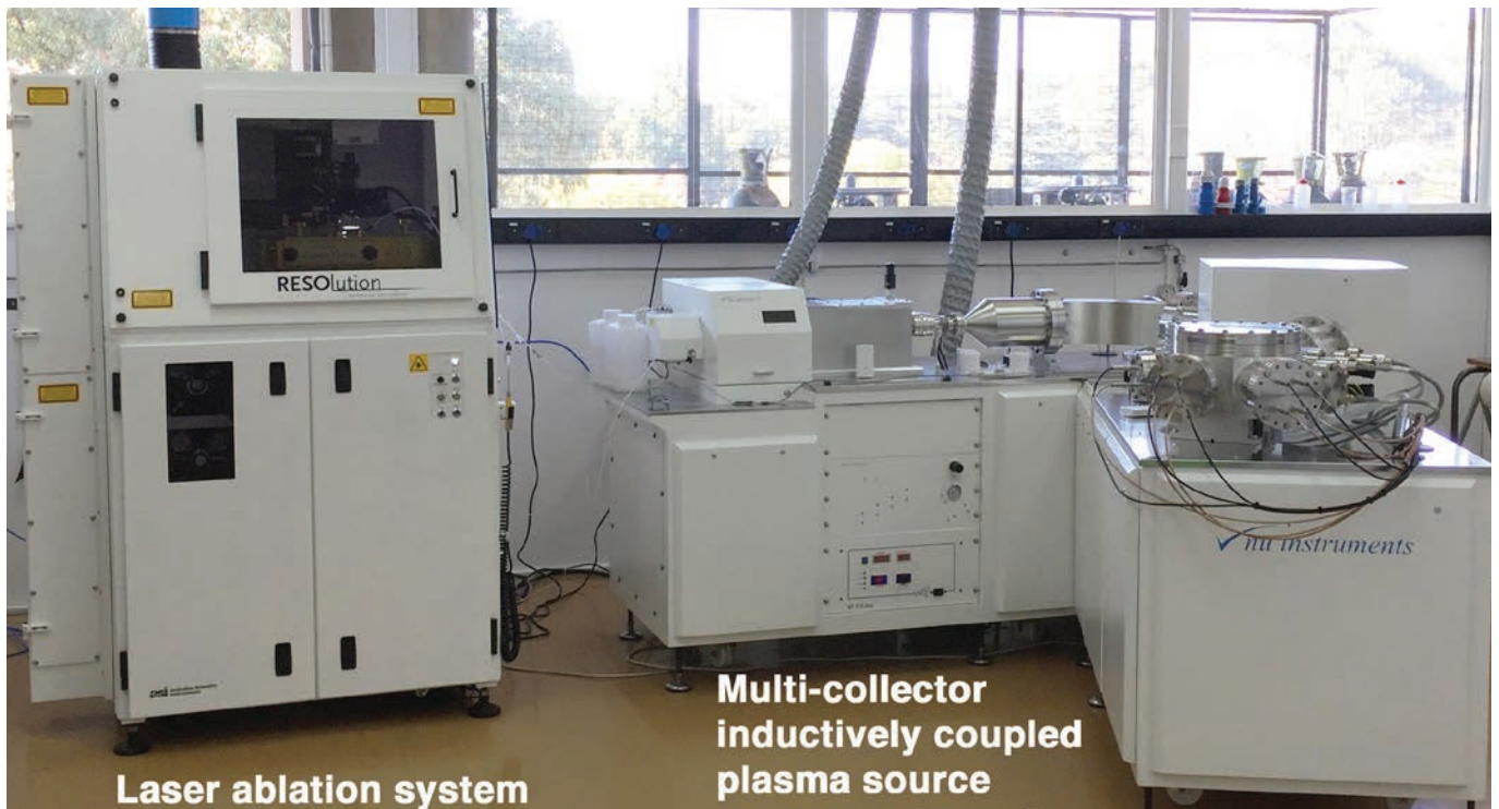
Fig. 1: Laser ablation system (ASI Resolution) and multi-collector ICPMS (Nu Plasma II) at the University of Johannesburg
